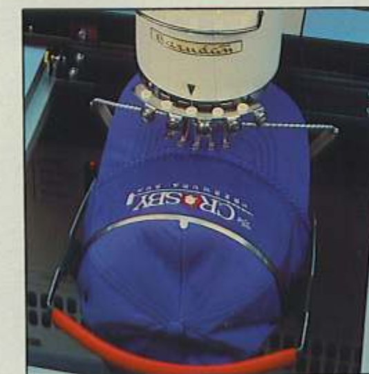
Embroider finished caps without distortion or puckering with Macpherson's cap frame.
